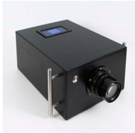
Dave Kemp, The One Pixel Camera , 2014, Wooden box, tripod mount, Zeiss lens, LCD viewfinder, custom electronics and software.
